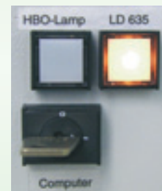
The PAS integrates an Ar-laser, red laser diode, and UV mercury arc lamp.
